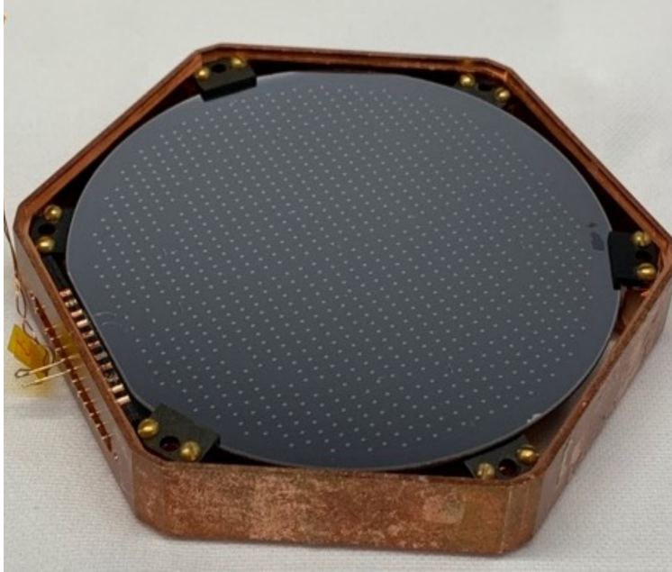
Figure 3.4: A picture of the CPD installed in a copper housing. The instrumented side is shown facing up.
