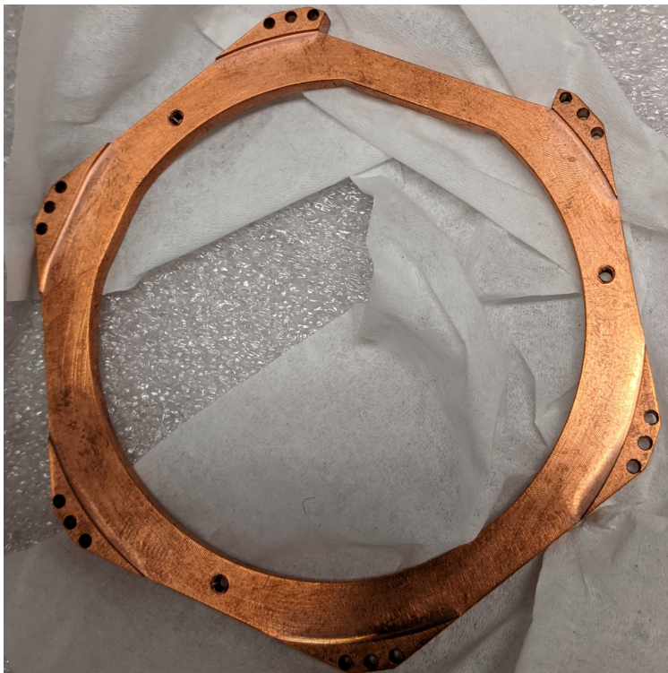
Figure 5.14: Stress free holder for the CPD for removal of stress-induced events, designed by Samuel Watkins. This holder will be used in a future run, and has not been run yet as of June 2022.
