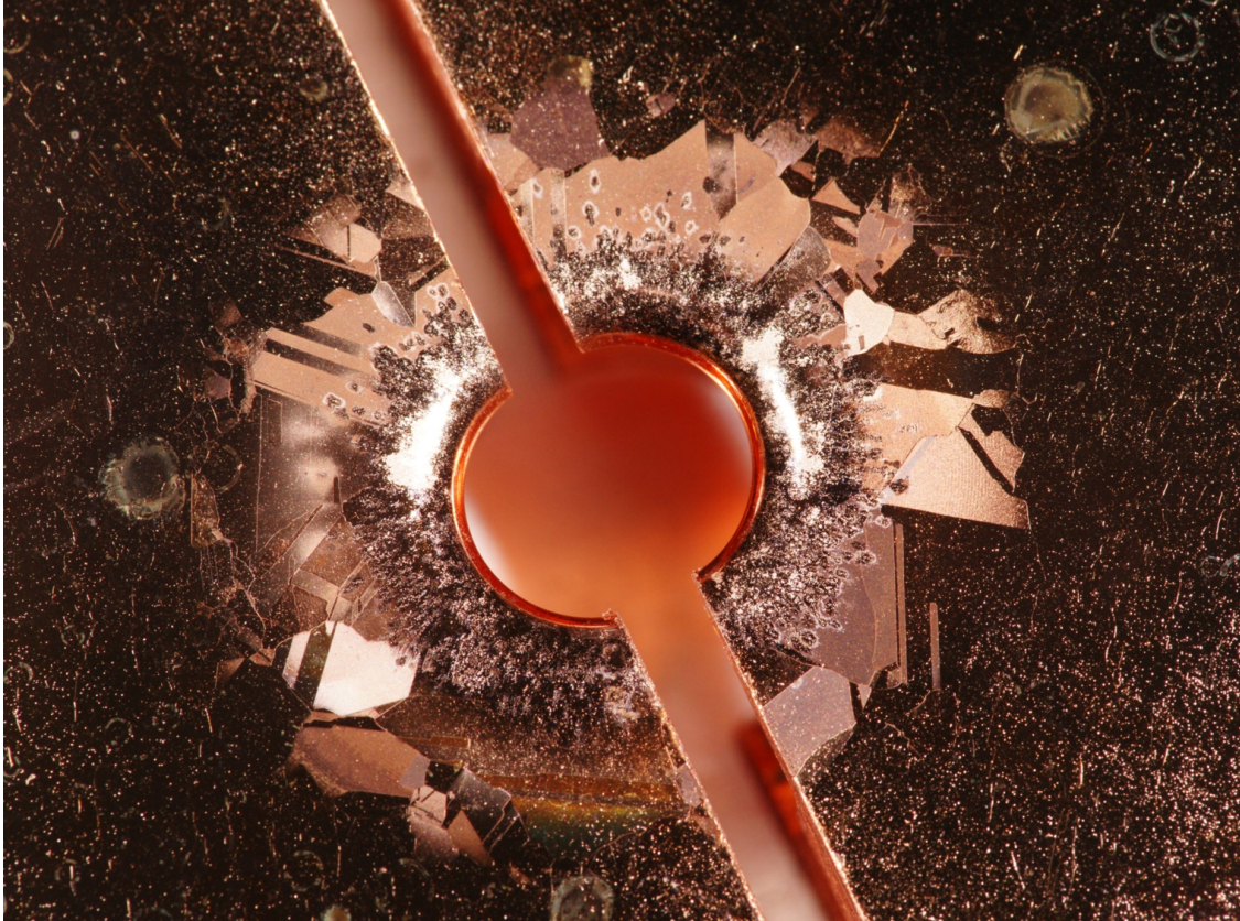
Figure 2.3: Photograph of the iris of a SW accelerating structure where damage is clearly visible due to breakdowns. The breakdowns occur in large field regions on the surface of the metal. Image Courtesy of [91]
