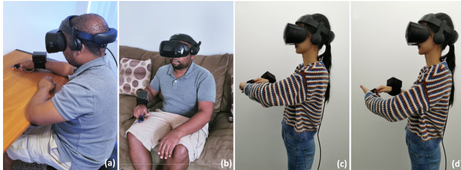
Figure 5.1: Two users using Shapeshifter to gesture type in VR in four scenarios: (a) on a desk when sitting down, (b) on the lap when sitting down, (c) on the back of the hand when standing up, and (d) on the palm when standing up. Both users are wearing the digital thimble introduced in this paper for gesture detection.
