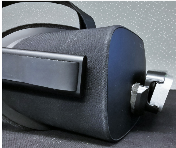
Figure 2.1: A Leap Motion Controller was attached to the front of the Oculus Rift at a 20° down angle to increase its field of view when the user’s head is upright.
