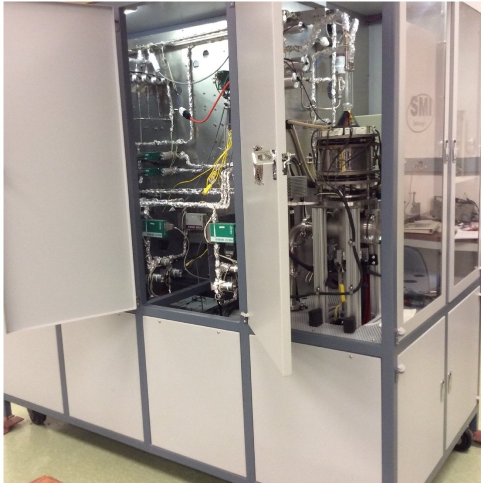
Figure 2.1 MOCVD installed at NECTAR Thin Films Lab, UC Santa Cruz.
