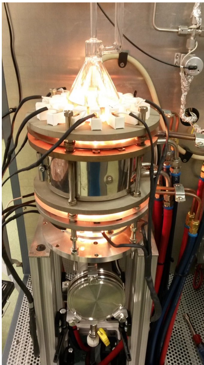
Figure 2.3 A photograph of the vertical MOCVD reactor chamber
