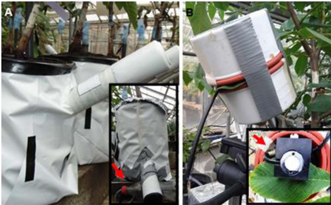
Fig. 1. Pots equipped with minirhizotrons tubes, on the weighing scales with the tensiometer and plastic reservoirs to collect the leached water (A); and a leaflet equipped with the psychrometer and the insulation capsule (B) Photo: Daniela Jerszurki.
