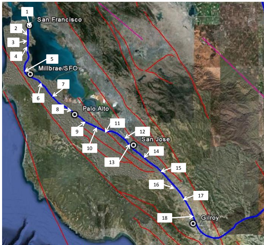
Figure 8.27: Ground motion prediction points along alignment
