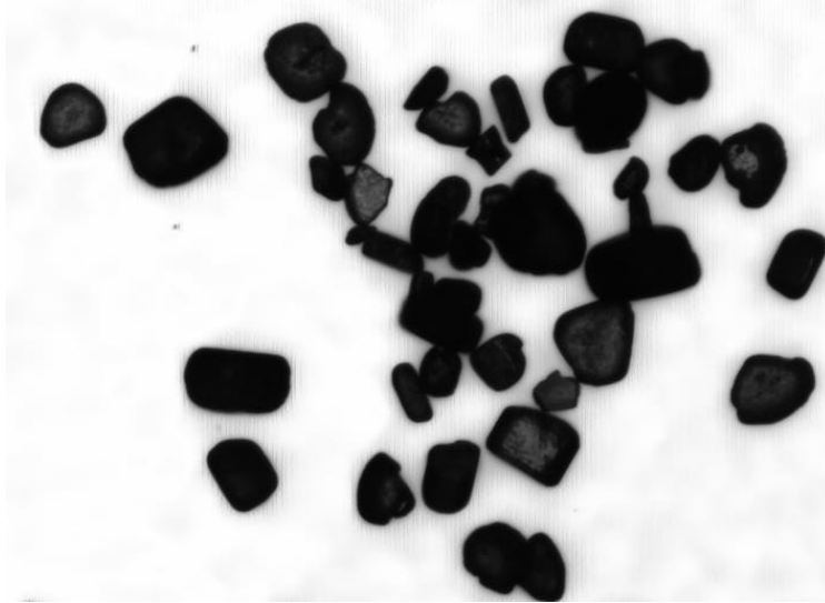
Figure 4.4. Microscope images of porous silicon particles after sonication.
