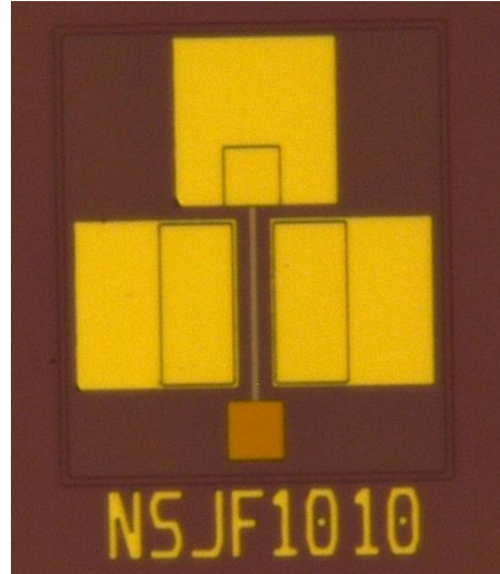
Figure 4.15: Optical image of a n-channel buried gate 4H-SiC JFET with L = 10 \mu\text{m} and W = 100 \mu\text{m} .
