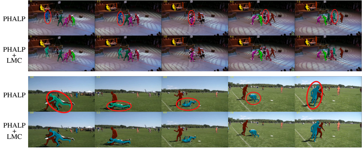
Figure 2.7: LMC results : We show to failure cases in our method. In the first example, MaskRCNN fails to detect the person (pointed in red) for long period of time. This causes the error in location prediction and therefore when this person detected again a new track is created. In the second example, HMR fails when the human pose is very different and causes a large cost in the pose distance. Due to this a new track is created for the same person. With LMC, we are able to look back and check whether these new track can be connected with any old tracks, and we connected them together as a single track.
