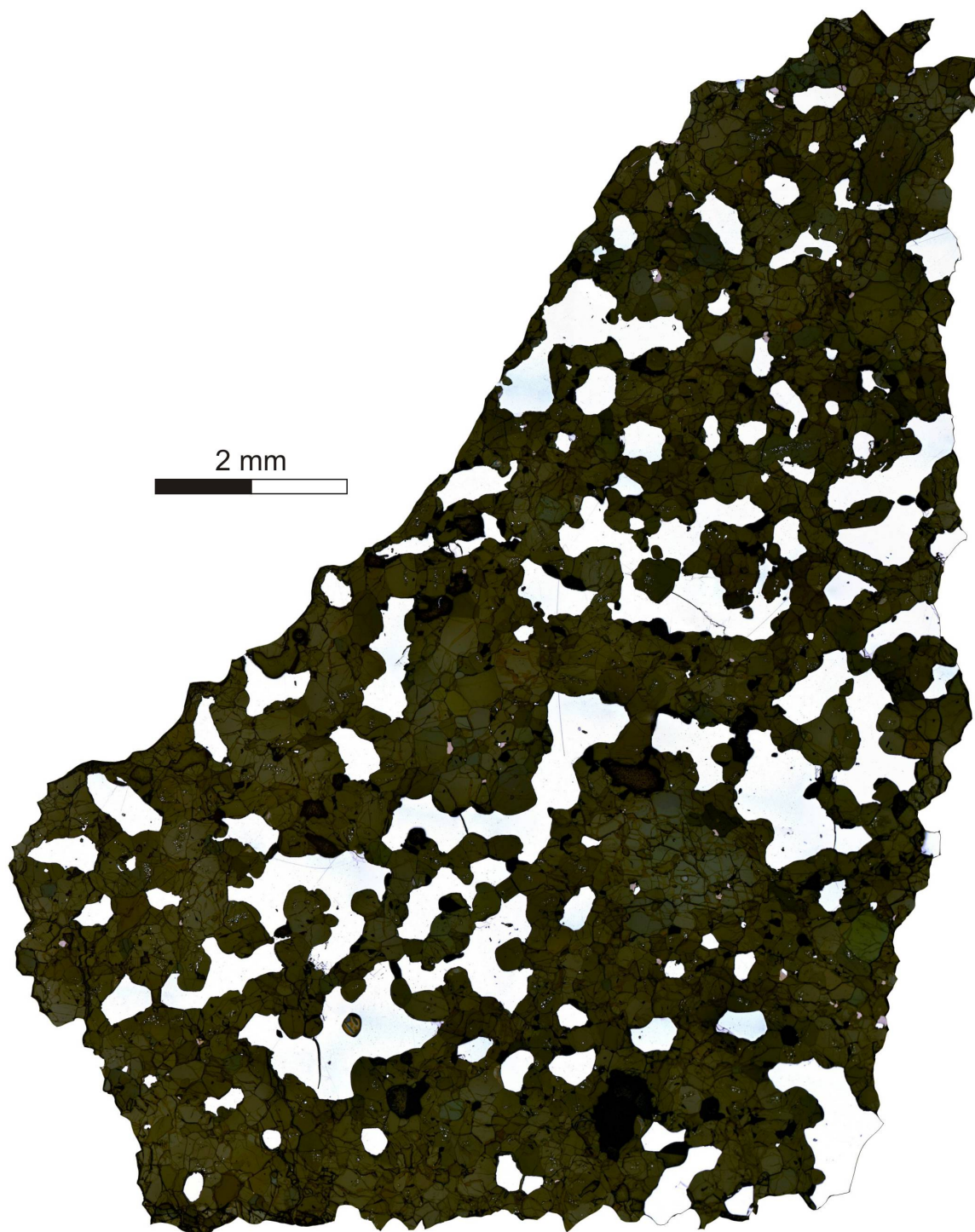
Figure 4.1.2: Reflected light photomicrograph map of the transitional acapulcoite-lodranite EET 84302, 28. This meteorite serves as a particularly useful demonstration of the migration of metal in primitive meteorites – the FeNi metal in this sample (large reflective minerals that appear white in this map) appears to have “pooled” into large anhedral grains.
