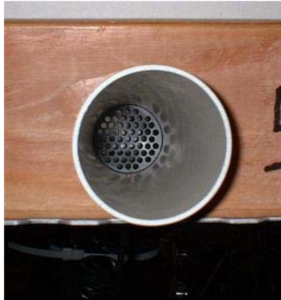
Figure 6. End view of boot leak showing the PVC plug used for the register closing tests.
