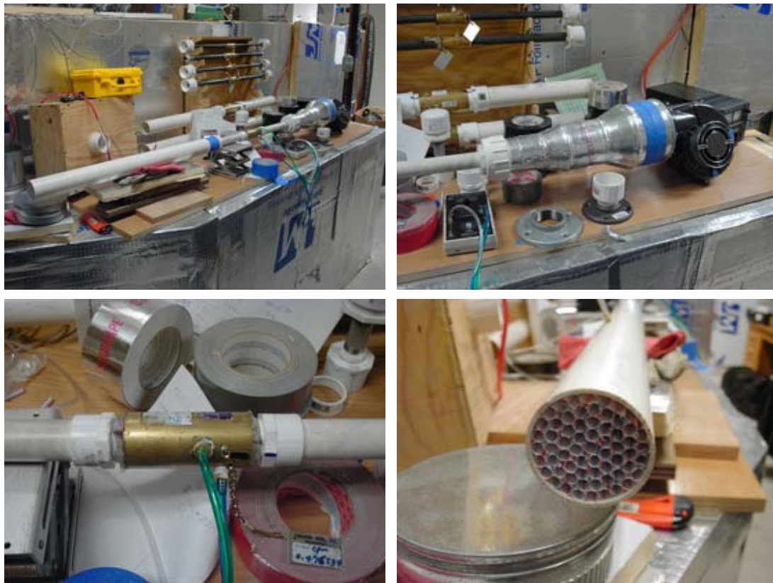
Figure A3. Calibration of boot leaks showing (clockwise from top left): complete calibration apparatus, variable speed blower and hand held manometer, high precision flow nozzle and end view of prototype boot leak filled with straws
