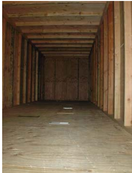
Figure A1. Photographs of test chamber construction showing registers located in the floor
