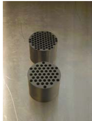
Figure A4. Construction of controlled pressure exponent boot leaks machined from solid PVC blocks.
