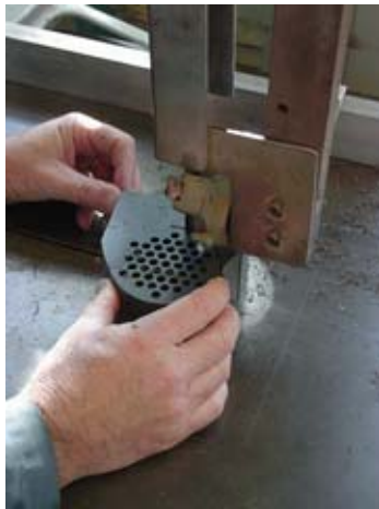
Figure A4. Construction of controlled pressure exponent boot leaks machined from solid PVC blocks.
