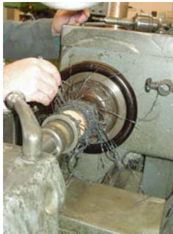
Figure A4. Construction of controlled pressure exponent boot leaks machined from solid PVC blocks.
