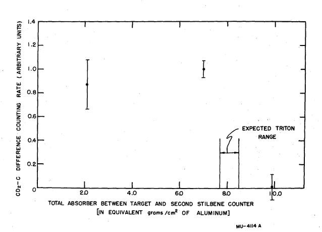
Fig. 8. Range spectrum of particles arriving at the triton counters, and causing a coincidence.
