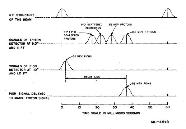
Fig. 5. Time sequence of particles arriving at the counters.
