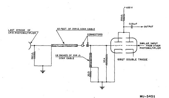
Fig. 3. Circuit used to shape, limit, and add photomultiplier pulses.
