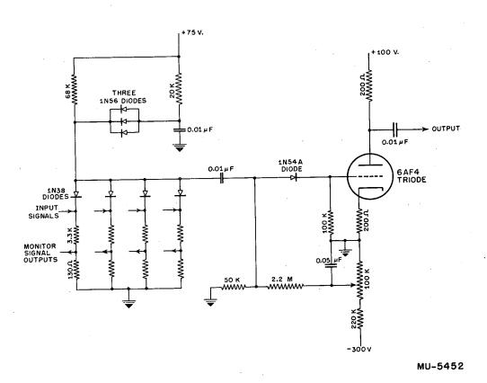
Fig. 4. Germanium diode quadruple coincidence circuit.
