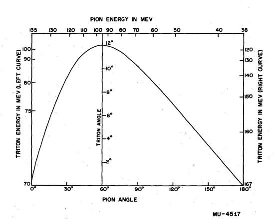
Fig. 1. Correlated angles and energies in the laboratory system for the process  $p+d \rightarrow t+\pi^+$ . The incident proton energy is 340 Mev.
