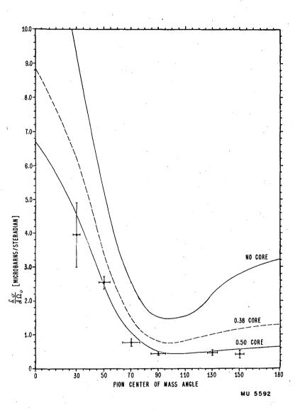
Fig. 10. Theoretical angular distributions for the process  $p+d \rightarrow t+\pi^+$ , compared with the experimental data.
