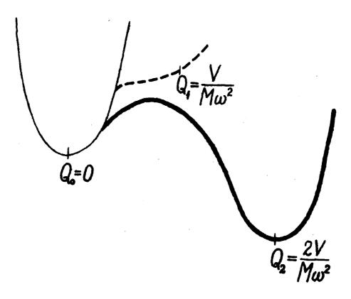
Figure 1: Proposed configuration coordinate diagramm for the DX center. The thin line shows the energy of the donor without electrons, the dashed line with one captured electron, the thick line with two captured electrons.  $Q_0$ ,  $Q_2$  are distortions corresponding to 0 and 2 captured electrons, respectively.
