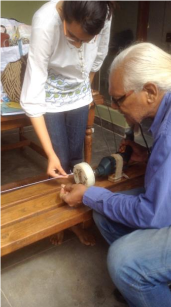
Setting up and using the Bradshaw cord maker (Photos by the author)
