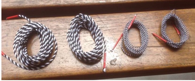
2, 4, 6 and 8 ply cords made using the Bradshaw cord maker (Photo by author)
