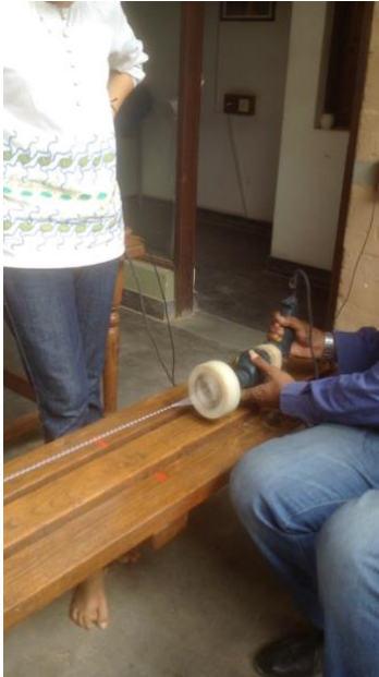
Setting up and using the Bradshaw cord maker (Photos by the author)
