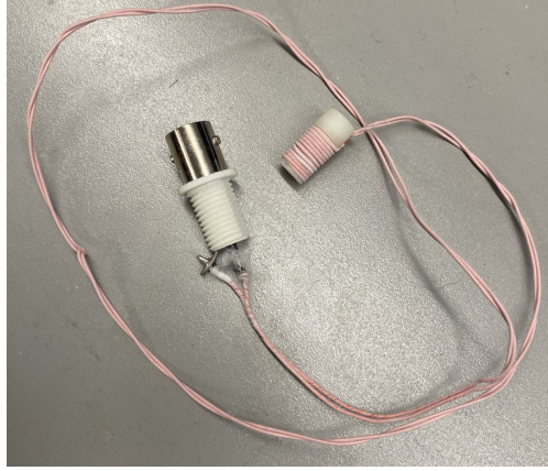
Figure 4.1: An example of a receive solenoid coil is pictured above. Typically receive coils for the AWR are litz wire solenoids to reduce the skin effect.
