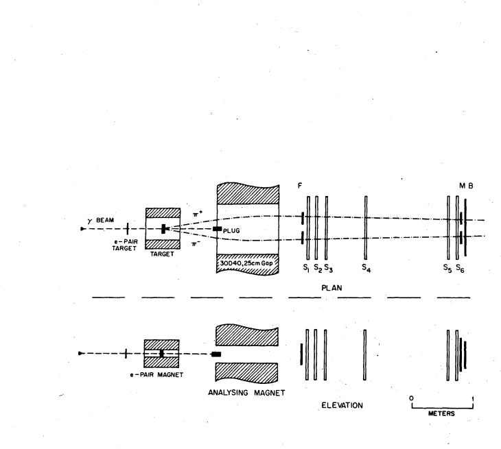
Fig. 3. Plan and elevation views of the experimental layout of the Rochester-Cornell-NAL group.
