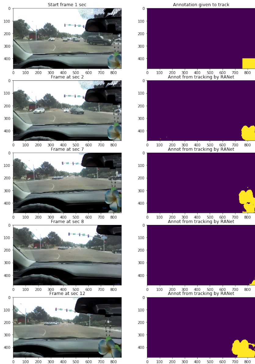
Figure 3.6. Tracking of a new class of object. A crude mask was generated on Frame 1 and given to RANet to track. This object was identified as car or road by HRNet (both non-adapted and adapted).
