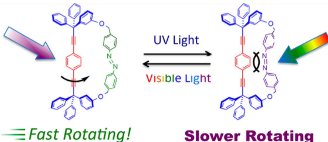
Figure 7. Azobenzene linked rotor exhibiting fast rotation in the trans form, after irradiation the azobenzene isomerizes to the respective cis form inhibiting the rotation from reference 31.
