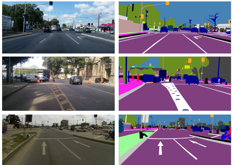
Figure 12. On the left we show images from the Mapillary dataset and on the right the visualized labels.
