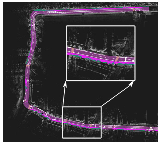
Figure 7. Generated map of testing data set in BEV, displayed on top of the dense point cloud map.
