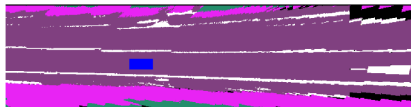
Figure 10. Semantic map generated by back-projecting 2D semantic image with a 3D planar assumption.
