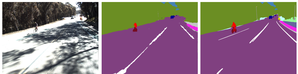
Figure 11. Semantic Segmentation Degradation from challenging lighting conditions. Left to right, original image, DeepLabV3Plus, MScale-HRNet.
