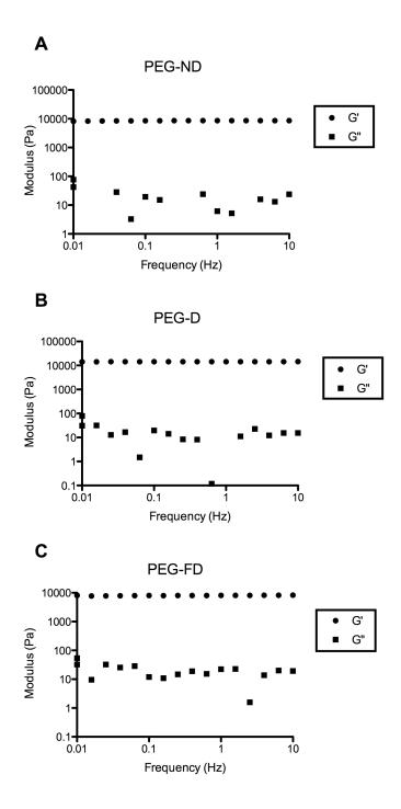
**Figure 3.1:** Mechanical spectra for PEG hydrogels. Typical mechanical spectra for a hydrogels formed by crosslinking of 4-arm PEG-ND (A), PEG-D (B) and PEG-FD (C) with 4-arm PEG-NH<sub>2</sub>.
