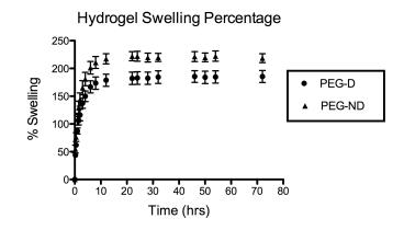
**Figure 3.2:** Hydrogel swelling percentage. Hydrogel swelling curve for (A) PEG-ND and (B) PEG-D hydrogels.
