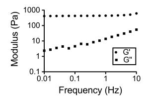
**Figure 2.1**: Mechanical spectra. Typical mechanical spectra for a hydrogel formed by crosslinking of 4-arm PEG-ND (100 mg/ml) and trilysine (1mg/ml).
