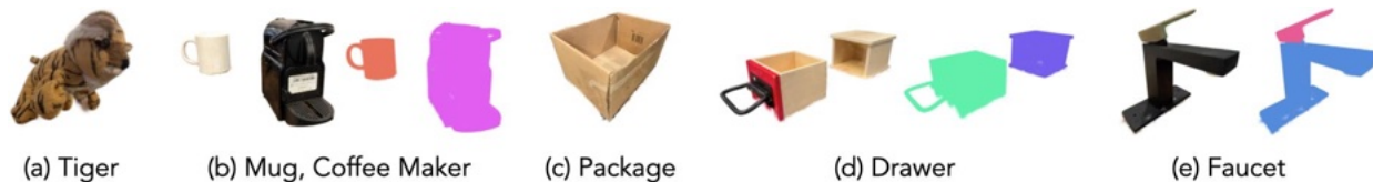
Figure 8.3: 3D Gaussian Splat Object Reconstructions with part-level segmentations derived from feature-based grouping. Objects are reconstructed and segmented into rigid or articulated components using GARField [337].
