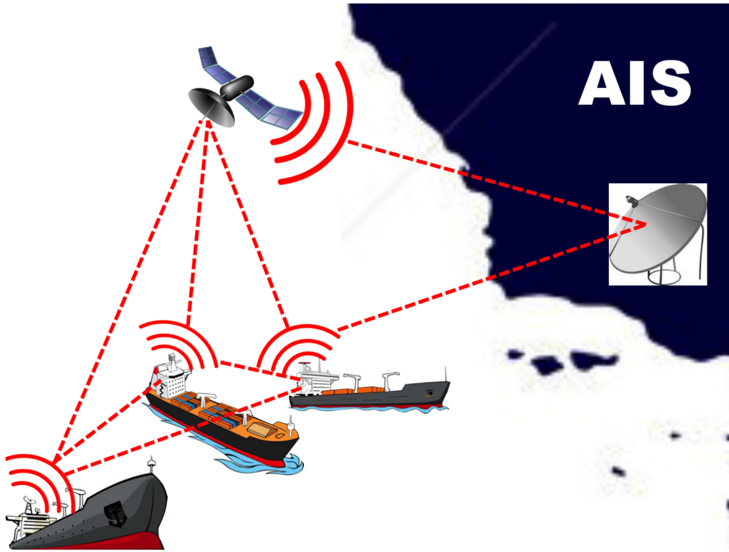
Figure 2.4: Cartoon depicting how AIS works. Each ship acts like a repeater for every other ship, significantly extending the range of the system. Also the transmissions from individual ships can be detected by satellites.
