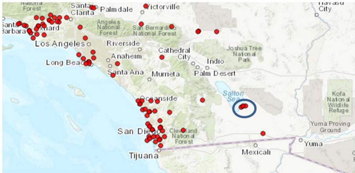
Figure 8.12. Map from NEI of point source H 2 S emitters in and around the Salton Sea and the SS-GF. Point sources are represented with red circles, and those circled in blue are geothermal plants in the SS-GF that report H 2 S emissions.
