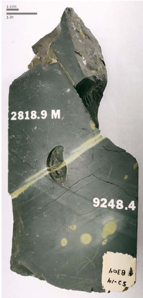
Figure A4.11. Epidotized mudstone from 2818.9 m (9248.4 ft) depth in the State 2-14 drill core.
