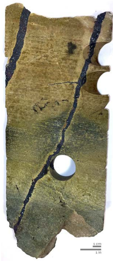
Figure A4.15. Metasedimentary mudstone with hematite veins from 1426.8 m (4681 ft) depth in the State 2-14 drill core.
