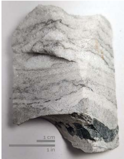
Figure A4.13. Interbedded anhydrite and mudstone from the Magmamax 2 drill core.
