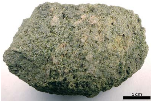
Figure A4.7. Monomineralic epidote from 1866 m (6122 ft) depth in the State 2-14 drill core.
