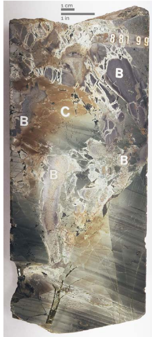
Figure A4.12. Brecciated diabase and mudstone from 2881.99 m (9455 ft) depth in the State 2-14 drill core.
