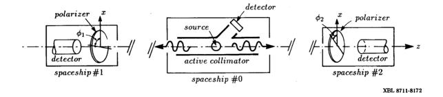
FIG. 1. Layout of an EPR-Bohm thought experiment: three spaceships and two photons (#1 and #2) with correlated helicities escaping spaceship #0. The events of interest are those events where a third photon (#0) has been detected in spaceship #0 but the active collimator did not detect any photon. Photons #1 and #2 will then fall on the polarizers in spaceships #1 and #2, respectively, and their plane of polarization will be analyzed by two observers posted there.
