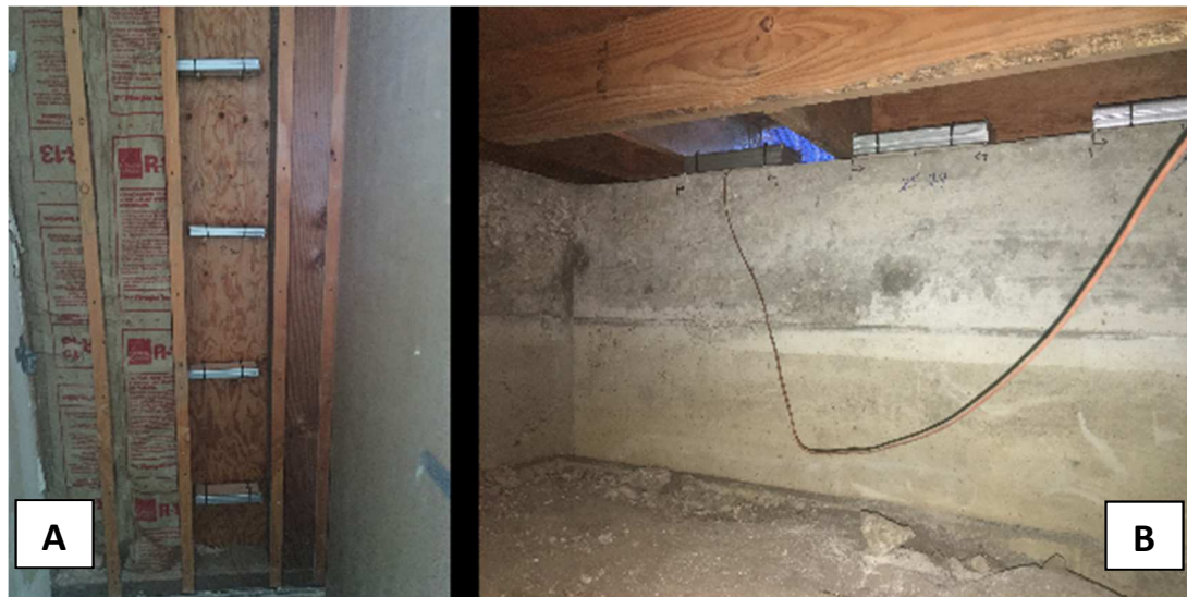
Fig. 3.3. Two different locations where the experimental arenas were placed. (A) Wall void. Brackets were used to place multiple arenas within a single wall void space. Four arenas are shown in the photo, and the bottommost one is a temperature monitoring arena. (B) Subarea. The arenas were placed on the top of concrete perimeter wall. The leftmost arena is a temperature monitoring arena.
