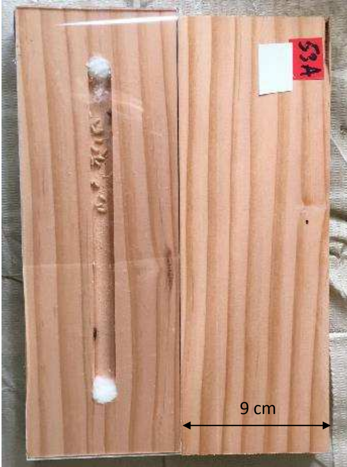
Fig. 3.1. Disassembled arena showing the top (right) and bottom (left) pieces of arena. A sheet of acrylic, the cotton balls, and termites inside the channel are shown on the bottom piece of the arena (left).
