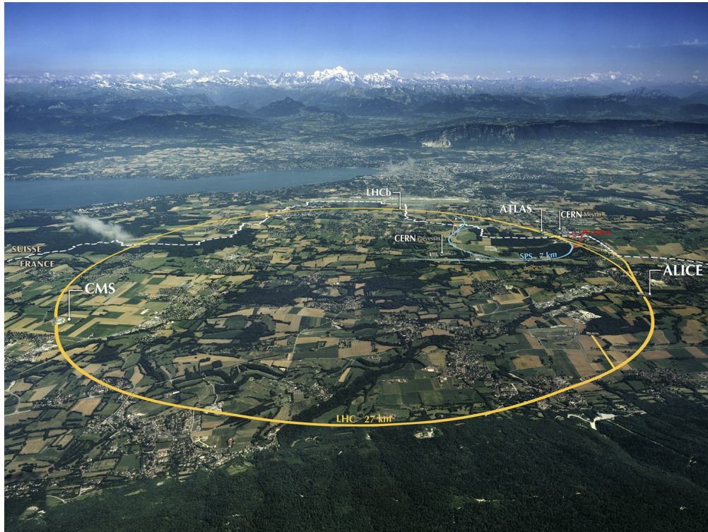
Figure 2.1. An aerial photo of the location where the LHC is buried [12]. The LHC ring is drawn in yellow, and smaller accelerators in the complex are in blue and red. The dashed white line indicates the border between France and Switzerland. Also labeled are the two main CERN laboratory sites, as well as the sites for the four main experiments.
