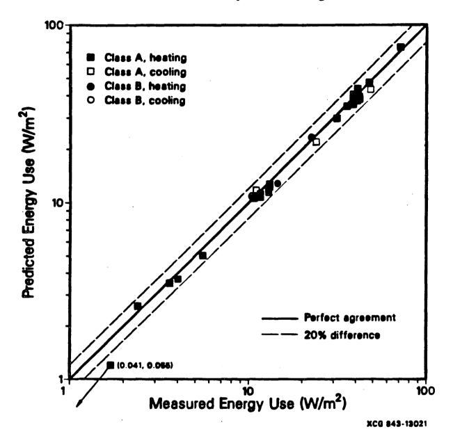
Figure 3. Average energy use over monitoring period for individual, unoccupied buildings. Detail of audit and consumption data (Class A = most detail, Class B = less detailed. None of these were Class C, least detailed) and enduses are indicated in symbol key. All simulations used weather data from the actual monitoring period, and were "blind" or with only verifiable errors corrected. Note log-log scale.
