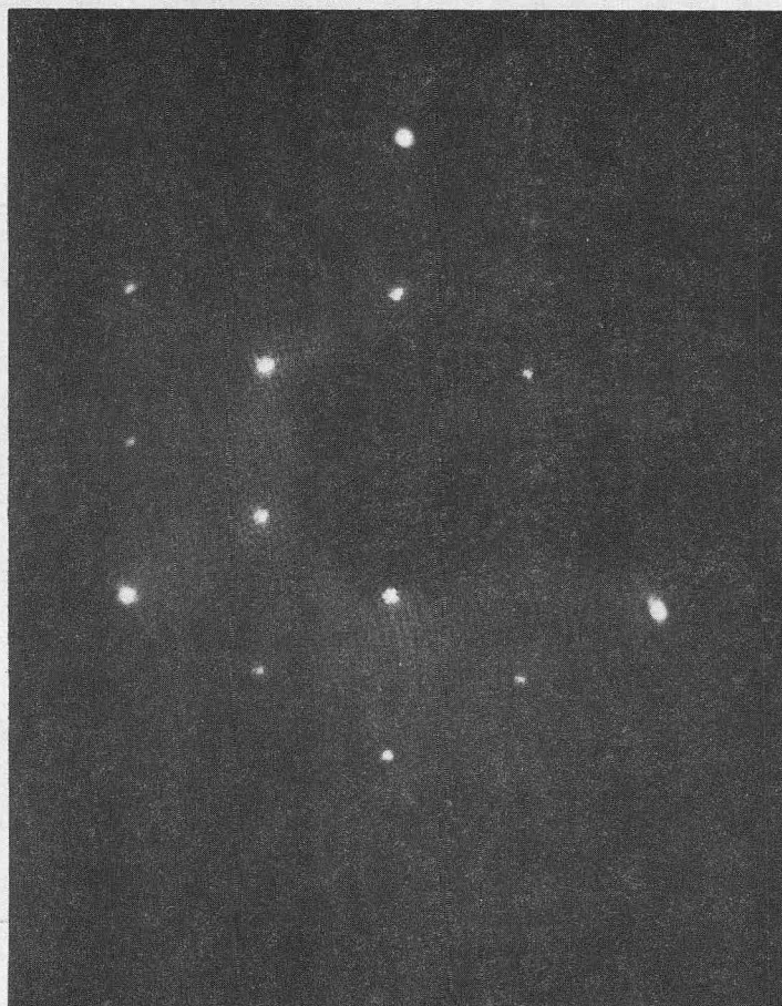
Figure II-6. LEED patterns of a clean Rh(111) surface and the same surface after exposure to C_2H_2 . In both diffraction patterns the incident electron beam energy is 68 eV.
