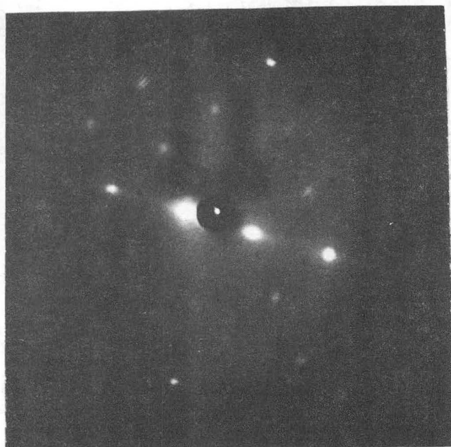
Figure III-33. (a) LEED pattern of \text{Rh}(331)-\begin{pmatrix} -1 & 1 \\ 3 & 0 \end{pmatrix} structure at 44 eV. (b) Real space unit cell of \begin{pmatrix} -1 & 1 \\ 3 & 0 \end{pmatrix} structure. A and B are \text{Rh}(331) unit cell vectors.
