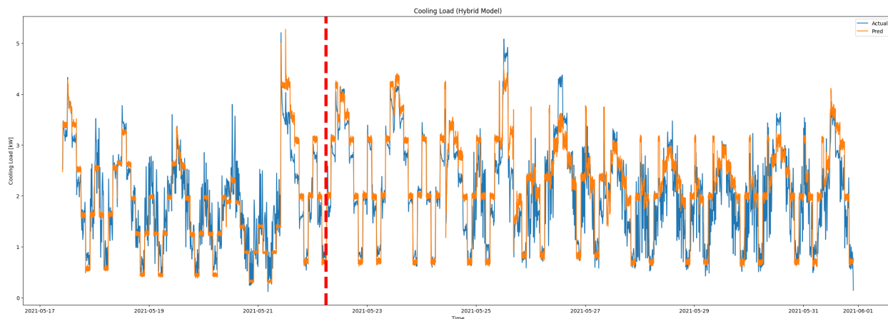
Figure 4.13: Comparison of measured and estimated cooling load data. The blue line represents the measured cooling load data, while the orange line represents the estimated cooling load data based on the hybrid model. The vertical red dotted line separates the calibrating (left) and validation (right) data.
