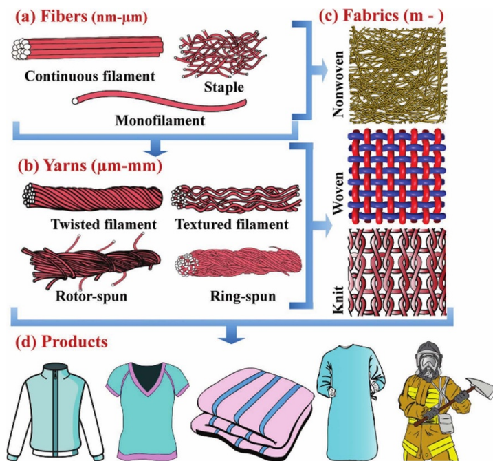
Figure 18. The structures of fibers, yarns, and textiles. [84] John Wiley & Sons. (Copyright © 2020 WILEY-VCH Verlag GmbH & Co. KGaA, Weinheim).
