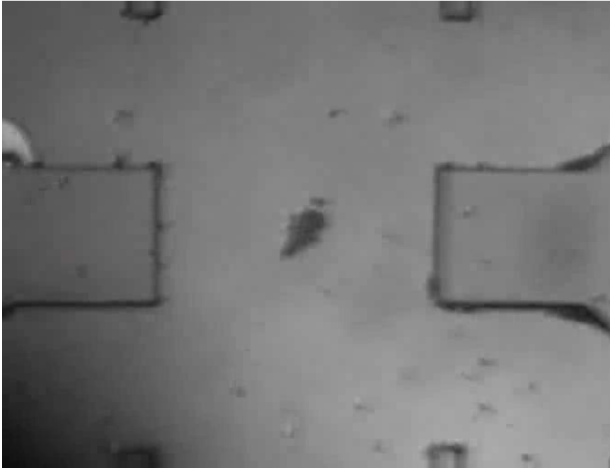
Figure 5.5: Optical image of 10 \mu\text{m} particles trapped in a structure similar to the one simulated in figure 5.4.
