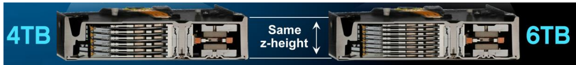
Figure 12: Size comparison between a Helium 7-disk HDD and an air 5-disk HDD[6]
