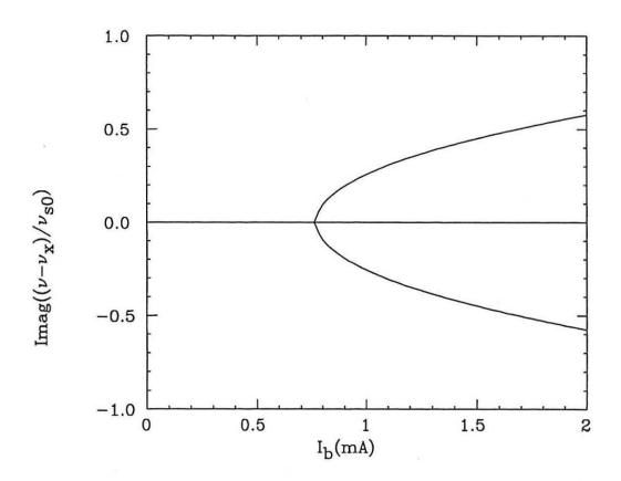
Figure 2: Imaginary parts of  $(\nu - \nu_x)/\nu_{s0}$  in the single rf system.
