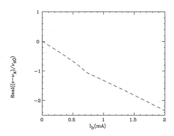
Figure 5: Real parts of  $(\nu - \nu_x)/\nu_{s0}$  in the double rf system.  $\sigma_{\phi}R/h = 10.8$ cm.
