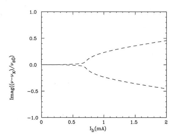
Figure 6: Imaginary parts of  $(\nu - \nu_x)/\nu_{s0}$  in the double rf system.  $\sigma_{\phi} R/h = 10.8$ cm.
