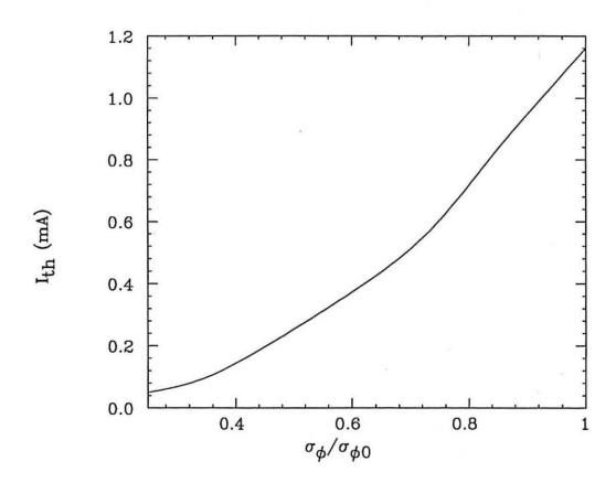
Figure 8: Threshold bunch current  $I_{th}$  as a function of the bunch length  $\sigma_{\phi}$  in units of  $\sigma_{\phi 0}$ .
