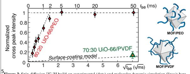
Figure 3: Spin-diffusion <sup>13</sup>C-<sup>1</sup>H build-up experimental (dots) and molecular dynamic simulation (lines); here t<sub>sc</sub> represents the mixing time for exchange.PVDF coats the surface of UiO-66; PEO interpenetrates the crystals as apparent by the build-up curves .Adapted from reference 33.
