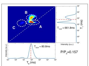
Figure 4. 2D relaxometry, in the form of a  $T_1$ – $T_2$  correlation map, presents three adsorbate populations for MeOH loaded into ZIF-8. (from reference 39).
