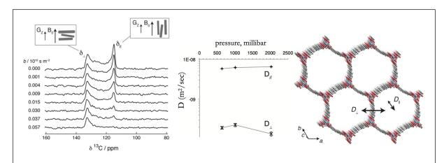
Figure 5. Residual chemical shift anisotropy of long-range diffusing  $^{13}\text{CO}_2$  was used to measure magnitude and directionality of diffusion. Left: the change in the  $\text{CO}_2$  NMR signal as a function of shift (crystallite orientation) and gradient strength b. Middle, the magnitude of self-diffusion along and perpendicular to the channel. Right: visualization for the pore channel in MOF-275.  $^{51}$
