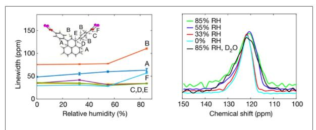
Figure 10: <sup>13</sup>C CP-MAS NMR spectroscopy of Al-PyrMOF, a MOF created to adsorb CO<sub>2</sub> at the exclusion of water. Left: c linewidths assigned to carbon sites A-F; Right: static spectrum of adsorbed CO<sub>2</sub> as a function of relative humidity.
