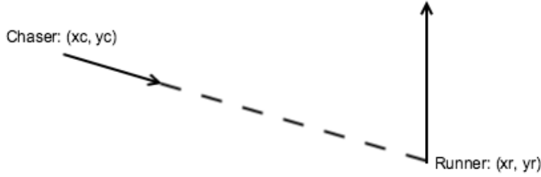
Figure 3.7: Diagram illustrating motion of runner and chaser. At any instant of time, the chaser's velocity vector points toward the runner's current position.
