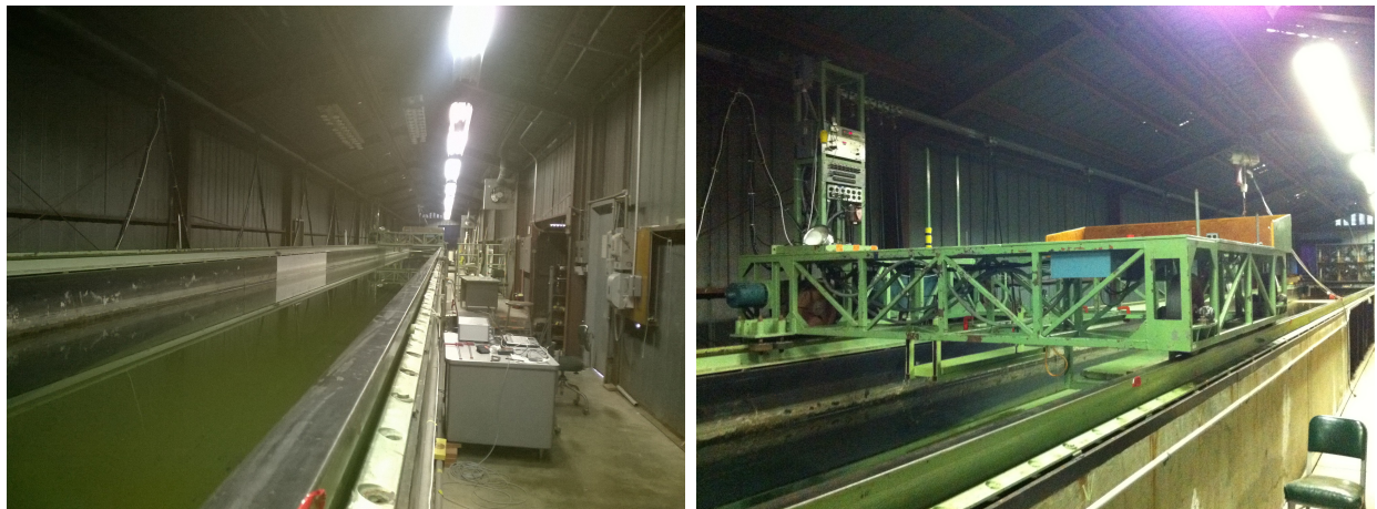
Figure 4.1: Towing tank and the carriage of Richmond-Field Station.
