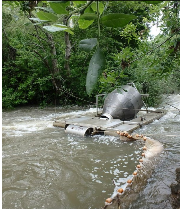
Figure 3. Lagunitas Creek Rotary Screw Trap. The drum of the trap faces upstream and the floating box at the back is where individuals are held prior to release. The trap is adjusted so that flows allow for the drum to spin between 3-8 revolutions per minute (RPM). In the event of high flows, the trap is disengaged to reduce smolt mortality. In the event of reduced flows, plywood baffles are installed upstream of the trap to direct flow into the drum to maintain RPMs. The rear of the trap is netted to maximize smolt capture.
