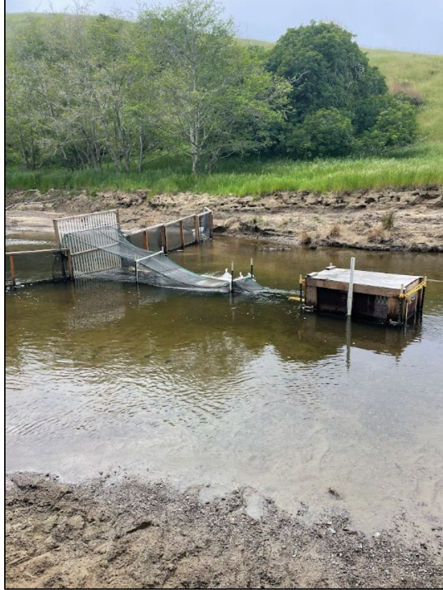
Figure 2. Walker Creek Smolt Trap. This picture shows the Walker Creek channel, spanned by a downstream migrant fyke net trap. A gap is maintained at the river left edge for migratory steelhead. The trap is operated by California Department of Fish and Wildlife staff and maintained daily for the duration of the season.
