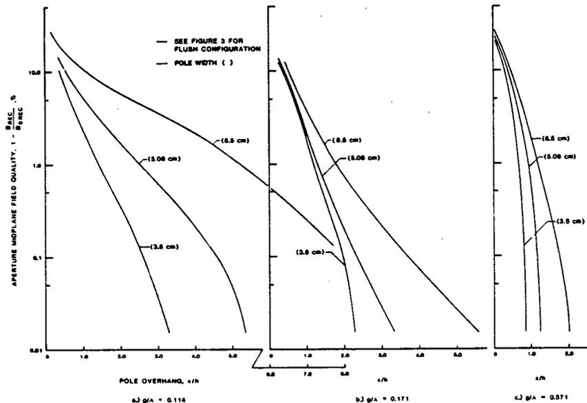
FIELD QUALITY AS A FUNCTION OF POLE OVERHANG FOR DIFFERENT WIDTH FLUSH CSEM-STEEL HYBRID CONFIGURATIONS
