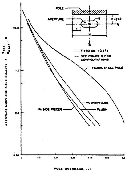
FIELD QUALITY AS A FUNCTION OF POLE OVERHANG FOR 8.5 cm WIDE POLE CSEM-STEEL HYBRID CONFIGURATIONS
