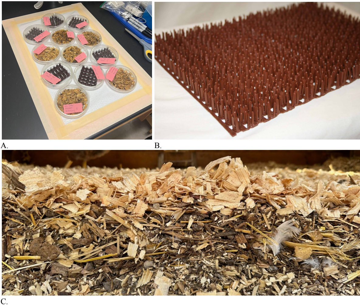
Figure 1. A. Experimental design with petri dishes, Litter, and Turf. B. plastic Turf material. C. Chicken Litter made up of wood shavings, straw, dirt, feces, and feathers.
