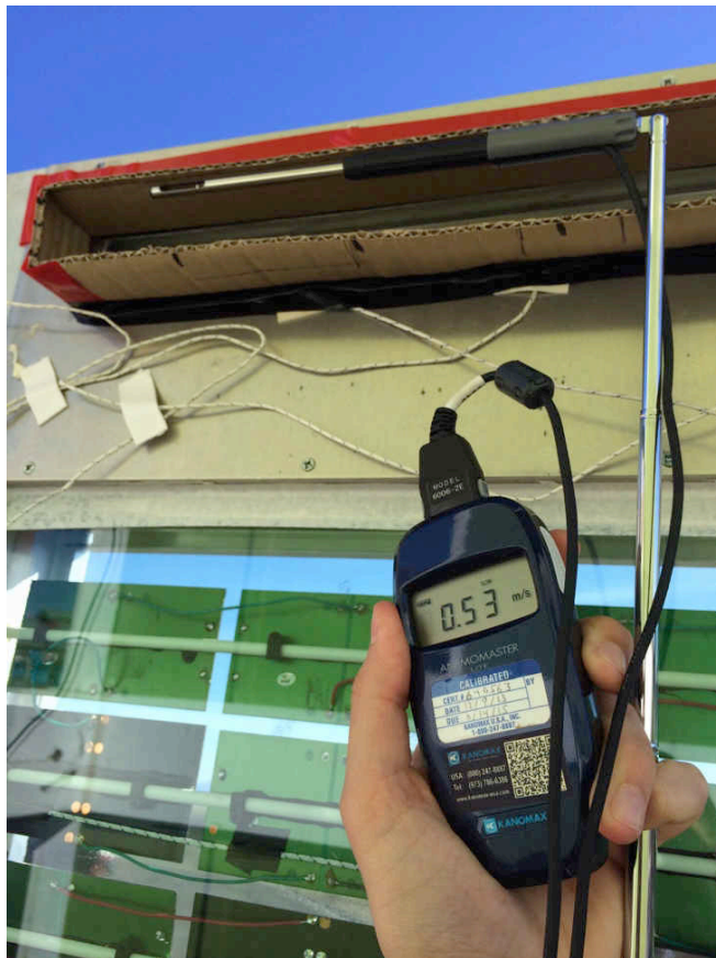
Fig. 4.3: Hot wire anemometer for air velocity readings.
