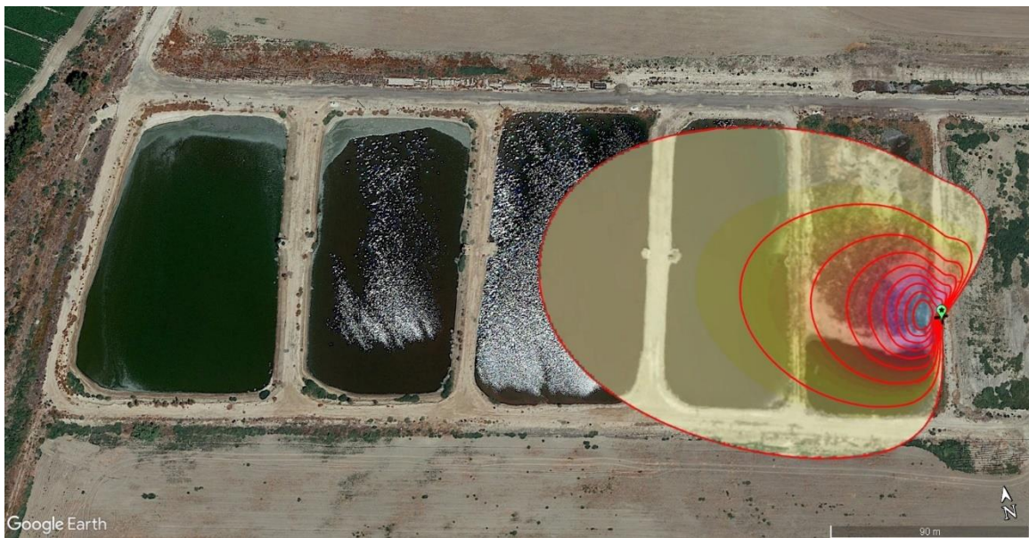
Figure 4.3. Flux tower area with footprint raster and contour lines from 10 to 90%, in 10% steps. Location of eddy covariance tower is indicated by the green symbol.
