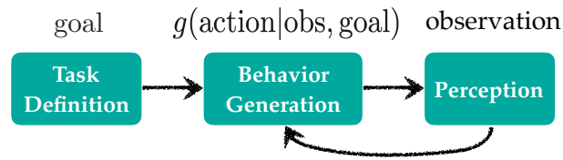
Figure 1.1: The three key elements of autonomous systems: the task definition module describes a set of tasks that the systems are designed to perform. It can either be as detailed as a sequence of points in space for a machine tool to follow, or as abstract as a high-level instruction such as “clean the dishes” for a service robot to perform. The perception module collects information from the surrounding environment. The behavior generation module is designed to automatically interpret the defined task and generate appropriate behaviors based on collected information in perception module.
