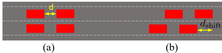
Figure 4.9: (a) The configuration without shifting distance in adjacent lanes. (b) The configuration with shifting distance.
