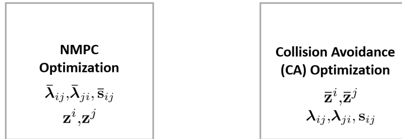
Figure 5.4: In NMPC optimization, the dual variables are kept fixed and in CA optimization, the primal variables are kept fixed.
