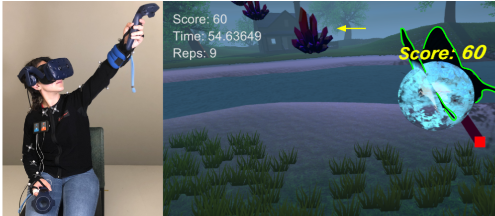
Figure 3.1: A participant is shown playing Project Butterfly using the HTC Vive. The silver dots on the player’s upper body are the reflective markers of the motion tracking system, and the blue strap on the arm is a wrist weight to help increase strength. The right-hand image is a capture from gameplay. The participant protects the moving butterfly, outlined in green, by placing the blue orb over the butterfly to protect it from the incoming crystals indicated by the yellow arrow.
