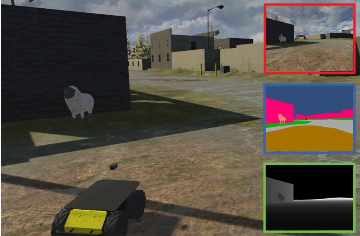
Figure 3.1. A robot autonomously explores an unknown environment using an RGBD sensor and a semantic segmentation algorithm.
