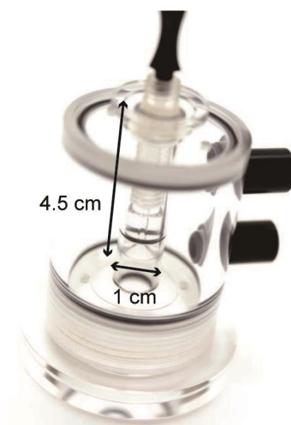
Fig. 7.3 Real image of the Clark electrode chamber. The diameter is 1 cm, and the height is 4.5 cm. Total capacity of this chamber is 2.5 mL.
