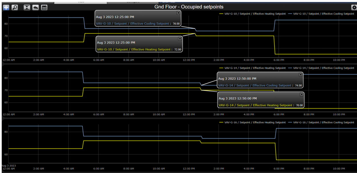
Figure 3: Trend output of setpoint correction in ALC in the courthouse field testing site
