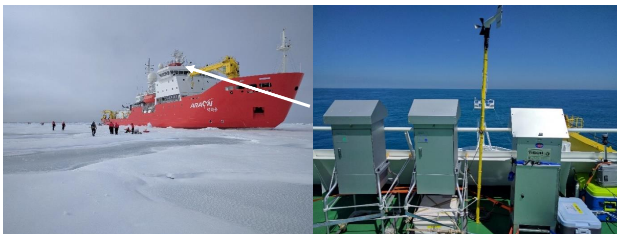
Figure 4.1 Picture of (left) R/V ARAON during ice camp activities and (right) high-volume sampling setup onboard the bridge deck. The white arrow points to the location of the sampler shown in (right).
