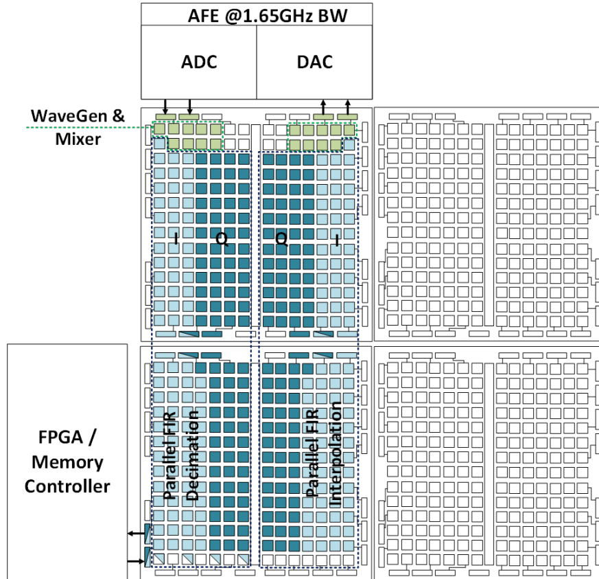
Figure 5.12: An example mapping of a digital up converter (DUC) and digital down converter (DDC) on the 2 \times 2 UDSP array, using digital mixers and 3-way parallel interpolation and decimation filters.
