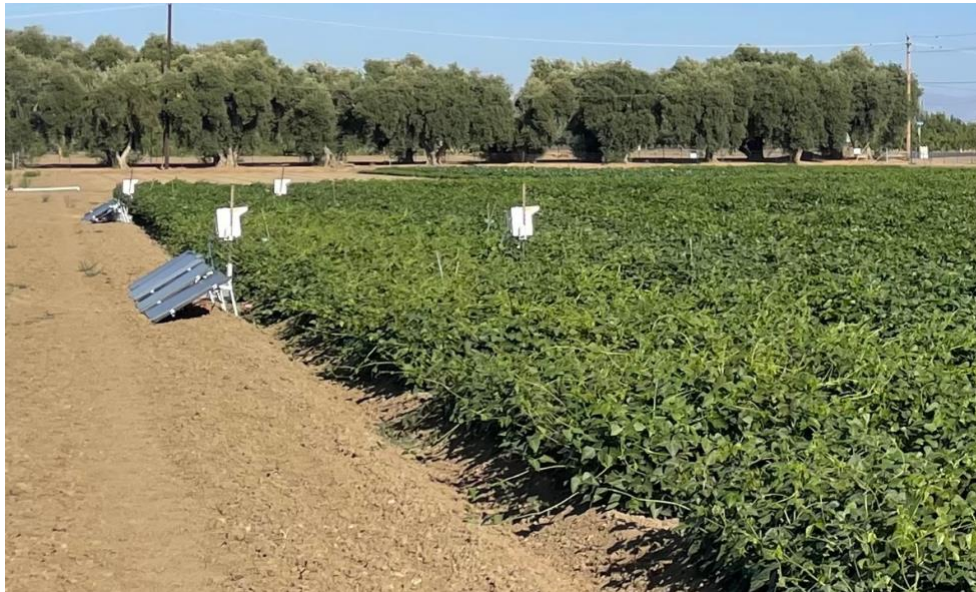
Figure 2: Autonomous near-infrared insect sensors (FaunaPhotonics ApS., Copenhagen SV, Denmark) installed over Lima Beans at the PSFF in June 2021. Data from the one sensor observing insects above the variety UC Haskell were used for this study.
